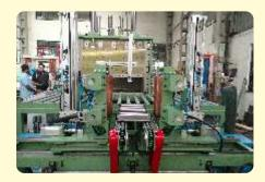
A welding machine to weld the side edges and to insert the reinforcing rod. The Machine consists of Conveyor with Automatic positioning , 2 torch carriages, Fin locking system and Control Panel.
